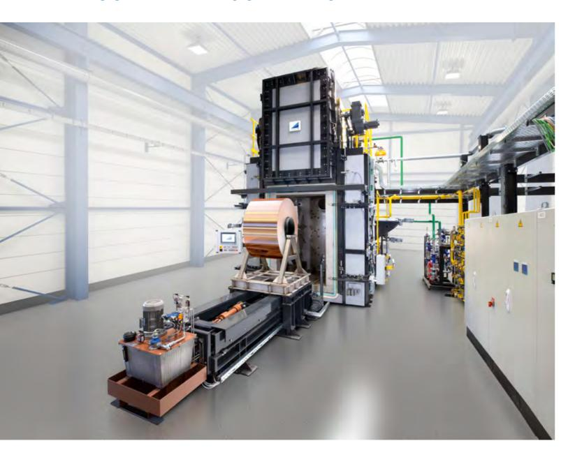
In addition to our heat treatment systems for press hardening and for heat treating aluminum, we also supply systems for heat treating **copper strips and coils** as well as **copper alloys** in the nonferrous metals sector.
