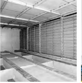
schwartz chamber furnaces serve to heat aluminum products of any geometry, from bulk parts in transport containers through ingots or billets to aluminum components arranged on trays.
