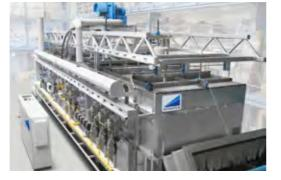
Our jet heating principle provides efficient heating via high-convection by recirculation air, flue gas or protective atmosphere. The gases are uniformly applied to the aluminum parts at high velocity by an array of nozzles adapted to the product. Due to the optimum nozzleto-product distance, a maximum heat transfer coefficient is achieved which is many times higher than with conventional forced air circulation – and the heat-up time is reduced accordingly.
