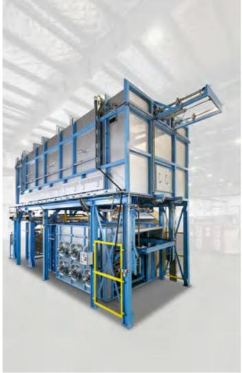
In a pusher furnace, the product is placed on trays and heated by a high-intensity recirculating airflow. Hydraulic pushers advance the racks through the heating chamber on skid rails according to the set pushing cycle. The loaded racks are fed into the furnace and discharged at the exit end by motor-operated elevators with chain transmission. Further space savings are achieved by placing the air-cooling zone underneath the furnace chamber.
