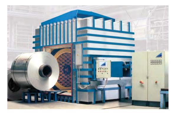
Jet rotation heating combines jet heating with a rotation of the nozzle banks. This patented system has been developed by us specifically for perfectly uniform heating of aluminum strip coils.
