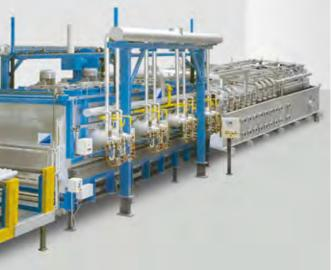
In our roller-hearth furnace for solution annealing, the aluminum rods and profiles are fed into the heating chamber appropriately spaced side by side on rollers. The heat treatment is carried out by high convection with the product resting on an oscillating roller track. Upon completion of the annealing process, the product is immediately fed into the attached high-pressure and low-pressure water quench, and finally, dried.
