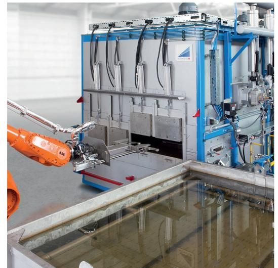
Exit end of solution heat treatment furnace for aluminum with robot and quenching tank
