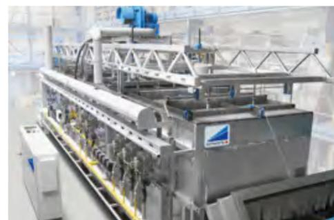
Our jet heating principle provides efficient heating via high-convection by recirculation air, flue gas or protective atmosphere. The gases are uniformly applied to the aluminum parts at high velocity by an array of nozzles adapted to the product. Due to the optimum nozzle-to-product distance, a maximum heat transfer coefficient is achieved which is many times higher than with conventional forced air circulation – and the heat-up time is reduced accordingly.
