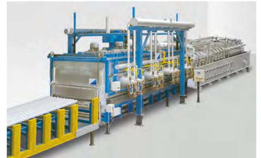
schwartz chamber furnaces serve to heat aluminum products of any geometry, from bulk parts in transport containers through ingots or billets to aluminum components arranged on trays.
