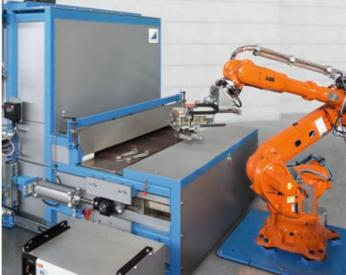
Robots also transfer the parts into the water quenching bath. Depending on your requirements, the subsequent aging process can be carried out either in our chamber furnaces or in our continuous or pusher-type furnaces.
