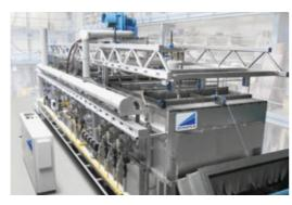
Our jet heating principle provides efficient heating via high-convection by recirculation air, flue gas or protective atmosphere. The gases are uniformly applied to the aluminum parts at high velocity by an array of nozzles adapted to the product. Due to the optimum nozzle-to-product distance, a maximum heat transfer coefficient is achieved which is many times higher than with conventional forced air circulation – and the heat-up time is reduced accordingly.
