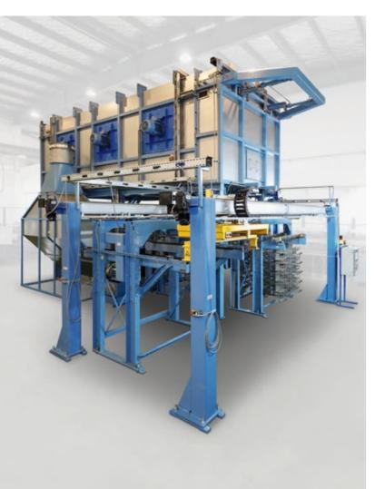
Apart from continuous conveyor furnaces, we also offer indexing pusher furnaces for artificial aging of forgings. These systems likewise provide fast and uniform heating, a quick return of parts into the processing workflow and, above all, substantially reduced space requirements.
