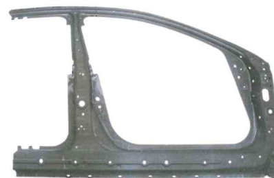
↑ Door ring heat-treated in a schwartz roller hearth furnace
