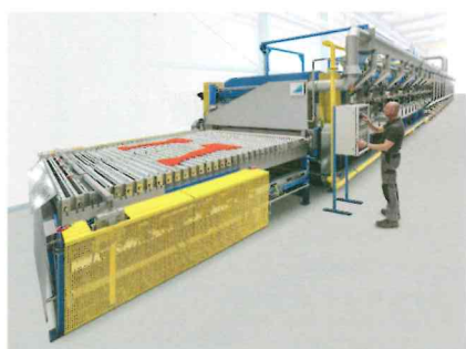
↑ Gas-heated roller hearth furnace for press hardening
