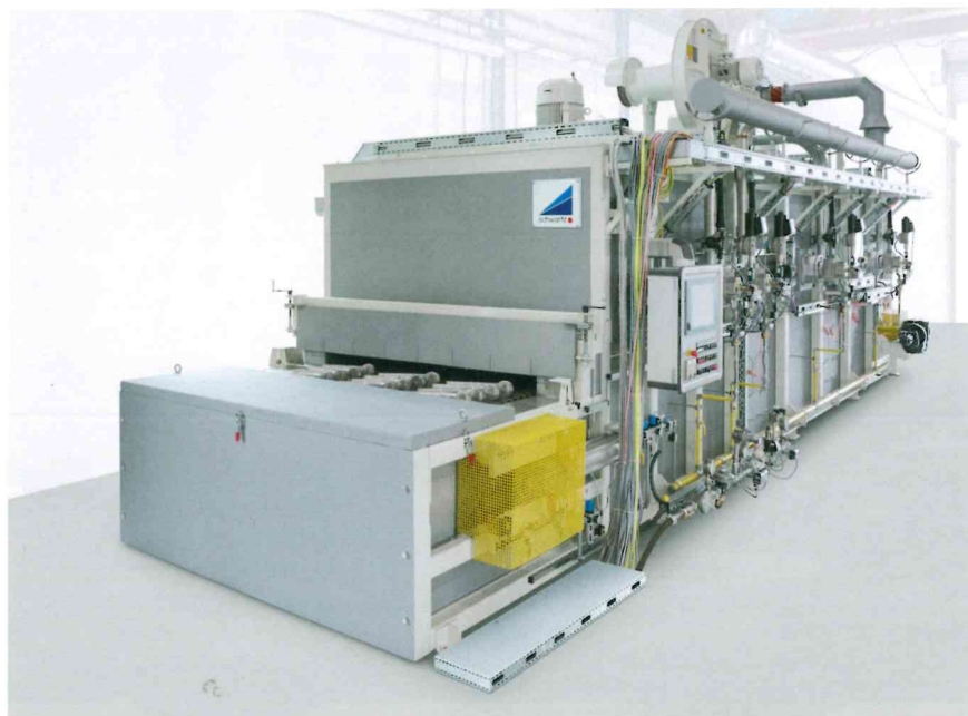
↑ Gas-heated heat treatment system for aluminum parts
